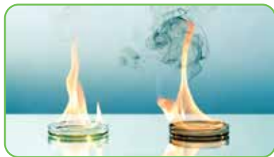
This image illustrates the cleanliness of HVO (left) in comparison to Kerosene (right), being burned.
